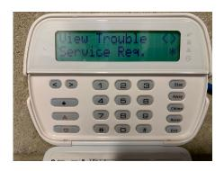
2. From this screen, press the star \* key again, and the keypad will tell you exactly what is wrong. In this example, there is a low back-up battery.
